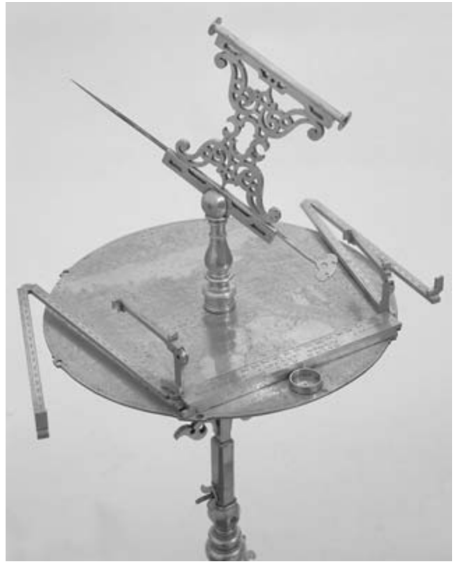
FIG. 19.17. EXAMPLE OF A SIGHTING TUBE ON A MULTI-FUNCTIONAL INSTRUMENT, 1557. On top of this multi-functional instrument, its maker, Baldassarre Lanci, fixed a sighting tube for better sighting with the additional help of a sharp pointer below. The round table that bears the sighting device is engraved with images of field surveying. Height of the tripod: 139 cm; diameter of table: 30 cm. Photograph by Franca Principe, courtesy of the IMSS (inv. no. 152, 3165).
