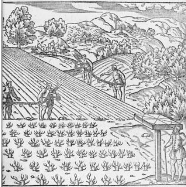
FIG. 19.19. MEASURING WITH A SIGHTING INSTRUMENT AND CHAIN, 1575. The sighting device (right) with straight grooves carved into the board substituted for the alidade. The use of chains hung on rods required very strong assistants, because the weight of the chain caused a sag that prevented accurate measurement of the straight-line distance. Size of the original: ca. 15.1 × 15.2 cm. Jean de Merliers, La pratique de geometrie descrite et demostree . . . (Paris, 1575), fol. A iij. Photograph courtesy of the BL (529.i.30).
