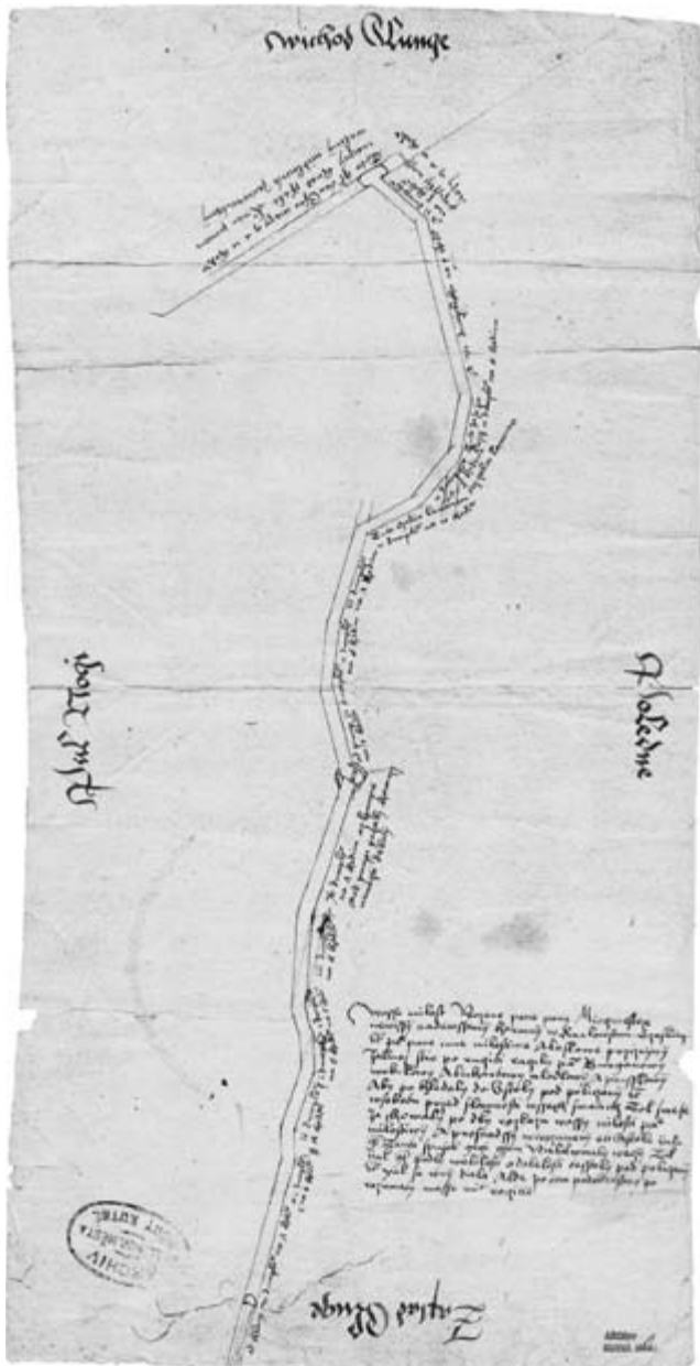
FIG. 19.5. OLDEST SURVIVING MINING DRAFT OF BOHEMIA NEAR KUTNÁ HORA (KUTTENBERG), DRAWN BY ZIKMUND PRÁŠEK, 1534. This schematic drawing depicts only one dimension of the gallery and is supplemented by verbal additions.
