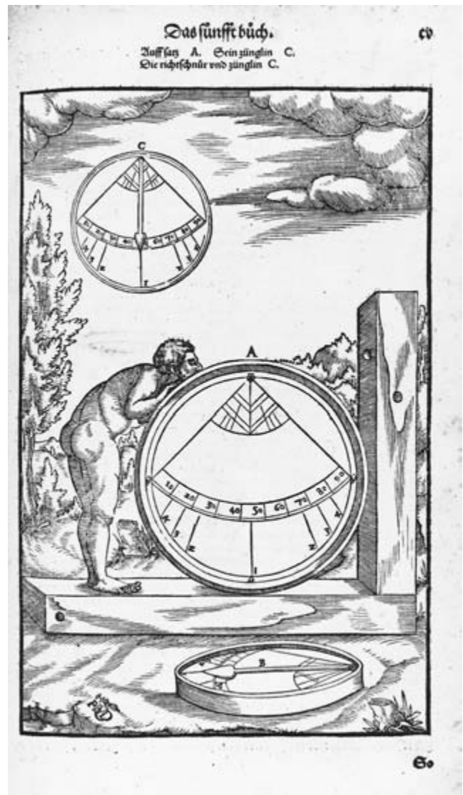
FIG. 19.7. MINE SURVEYING INSTRUMENT, 1557. A large quadrant with plumb bob is mounted into a circular frame to permit measurements of slope.
