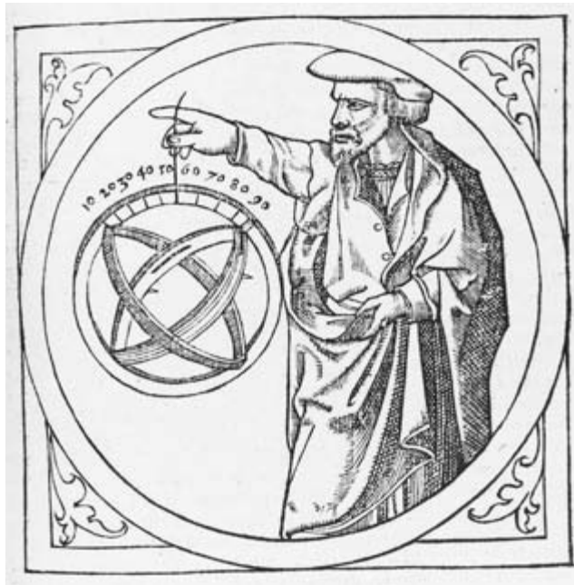
FIG. 19.16. ASTRONOMICAL RING INSTRUMENT FROM GEMMA. The astronomical ring consists of three metallic rings that bear a scale of degrees, from one degree to ninety degrees, for a quarter of the circle. The scale allows the observation of the stars and of the moon by night and also allows all sorts of land measurements. The shadows of the two thorns on one of the inner rings allow the observer to determine the height of the sun without damaging the eyes. A loop of rope allows the observer to hang the ring at his latitude (fifty-five degrees, shown in the example, is the latitude of Gemma's university town, Louvain).
