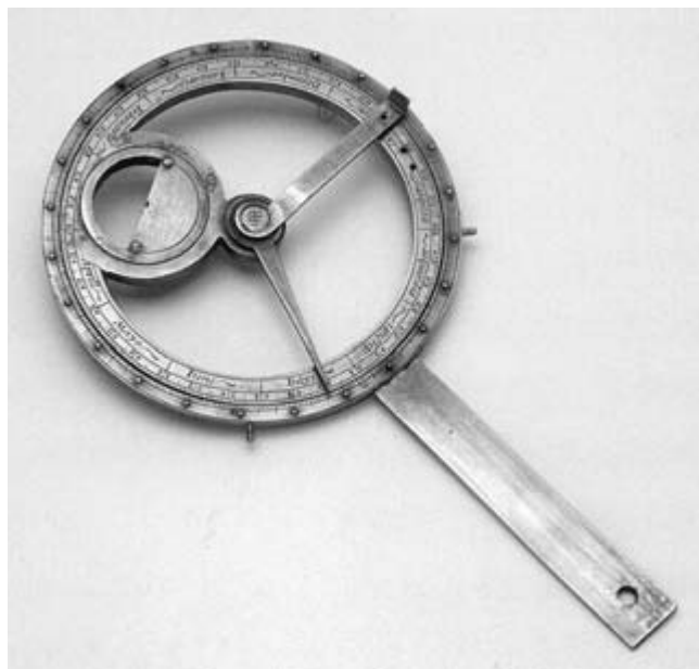
FIG. 19.9. ENGLISH NOCTURNAL, CA. 1600. The modifications to this instrument minimize the observational errors that originate in the daily and annual movements of Ursa Minor around the Pole Star, which does not precisely mark the north pole. Size of the original: 7.7 cm diameter. Photograph by Franca Principe, courtesy of the IMSS (inv. no. 2500).
