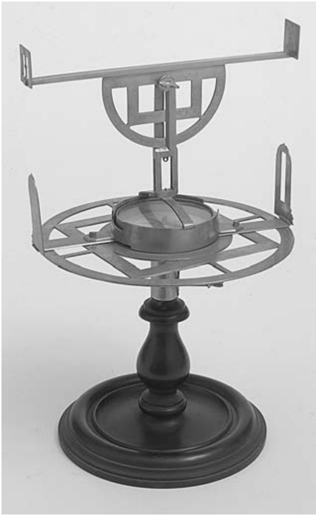
FIG. 19.15. ENGLISH THEODOLITE, 1590. Augustine Ryther's theodolite can be turned vertically (here the semicircle functions as a protractor) and horizontally (the circle also functions as a protractor) and has a magnetic compass at its center. The top balance is fitted with alidades, and shadow squares are incorporated into the circles. Size of the original: 23.5 cm diameter. Photograph by Franca Principe, courtesy of the IMSS (inv. 240).
