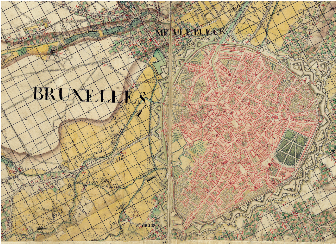
FIG. 237. DETAIL FROM THE FERRARIS CARTE DE CABINET, 1771–78, MADE FOR THE IMPERIAL GOVERNMENT IN VIENNA. The grid used in the field plans in preparation for copying to the assembled work is shown.
