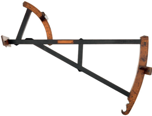
FIG. 398. AN UNSIGNED ENGLISH BACK STAFF, OR DAVIS QUADRANT, CA. 1700. The frame is made from lignum vitae , the arcs and vanes from boxwood, the fittings from brass. The sight vane was originally equipped with a Flamsteed lens (now missing). The sixty-degree or shadow arc (upper left) is graduated in 1^\circ intervals from 0^\circ to 65^\circ ; the thirty-degree or sight arc (right, with carved grip) has a transversal scale from 0^\circ to 25^\circ in 5' increments that can be read to 1' . Size of the original: 1.7 \times 67.2 \times 36.0 cm. © National Maritime Museum, Greenwich, London (NAV0045). The Image Works.
