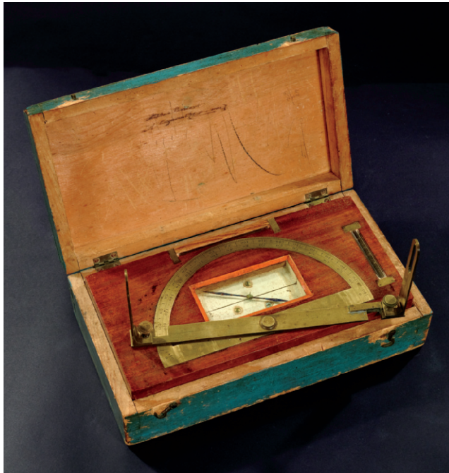
FIG. 408. A COLONIAL GRAPHOMÈTRE IN ITS PINE CARRYING BOX. Made in Boston, ca. 1775, this instrument served as a compact equivalent to the circumferentor. Such colonial instruments had trench compasses for orientation, two spirit levels, and a brass semicircle and alidade, all generally set into a wooden base. Here, the simple north arrow on the compass card is in manuscript, and the base is mahogany. Size of the original: 30.5 \times 15.0 cm; diameter of brass alidade and measuring limb: 22.7 cm. Image courtesy of the Osher Map Library and Smith Center for Cartographic Education at the University of Southern Maine, Portland (OS-1775-29).
