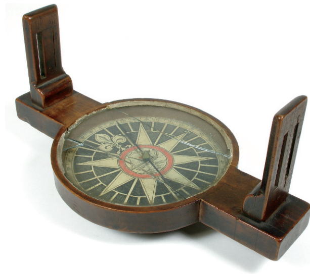
FIG. 400. JOSEPH HALSY, CIRCUMFERENTOR, BOSTON, 1747. Samuel Lane, a New Hampshire surveyor, acquired this instrument in 1747 and used it until it was damaged in 1754. The thick sights with two apertures each permitted the surveyor to take back sights without reversing the instrument. The compass card was printed from a woodblock and hand colored. Wood with glass face.
