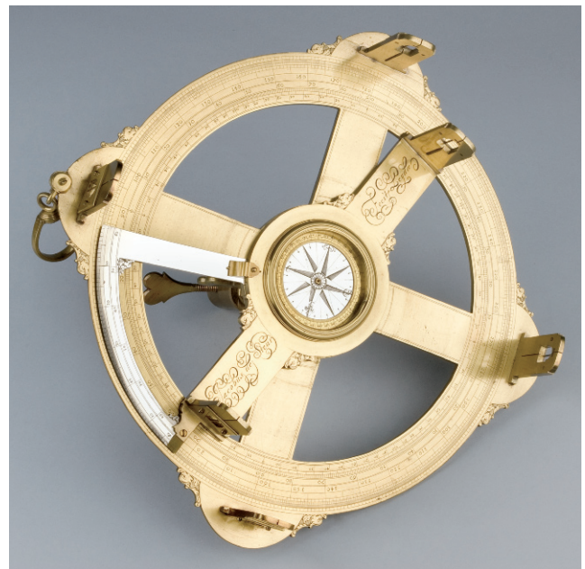
FIG. 405. HOLLAND CIRCLE BY JACOBUS DE STEUR, LEIDEN, CA. 1670. The outer circle of this brass instrument is graduated to fifteen minutes; the inner circle was marked with scales useful to military engineers. It came supplied with several attachments, including a sighting bar that can fit over the sights on the alidade. Size of the original: 6.2 × 32.6 × 36.0 cm. Image courtesy of the Collection of Historical Scientific Instruments, Harvard University, Cambridge (Inv. # DW0674a).
