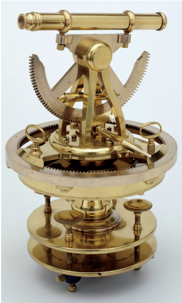
FIG. 409. EARLY THEODOLITE BY JONATHAN SISSON, 1737. The 6.5-inch (16.5 cm) diameter horizontal circle and 5.5-inch (14 cm) diameter vertical arc were both graduated to one-degree increments and both were equipped with vernier scales. The brass instrument was housed in a large octagonal wooden box. The telescope is a modern replacement. Size of the original: 17.0 × 16.3 cm. © National Maritime Museum, Greenwich, London (NAV1451). The Image Works.
