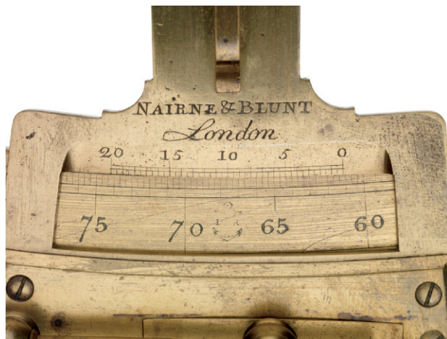
FIG. 402. DETAIL OF THE VERNIER SCALE ON A SEXTANT. The main arc (here showing from 75^{\circ} to 60^{\circ} ) is graduated in intervals of 20 minutes of arc; the vernier scale, above, permits those 20 minutes of arc to be read to a precision of half a minute, or 30 seconds of arc. The vernier scale moved with the sextant's telescope, with the final precise adjustment being made by a finely tuned screw (not shown here; see fig. 404). To read the angle, the mariner looked for the exact coincidence of one mark on the vernier scale with another on the main scale; here, the coincidence is between 65^{\circ}0' on the main scale and 6'0'' on the vernier, for a final value of 65^{\circ}6'0'' . Brass sextant made in London by Edward Nairne and Thomas Blunt, ca. 1780; the engraved mark on the main scale indicates that the circle was divided on Jesse Ramsden's dividing engine. Size of the original: 38.0 \times 35.8 \times 11.0 cm. © National Maritime Museum, Greenwich, London (NAV1110). The Image Works.
