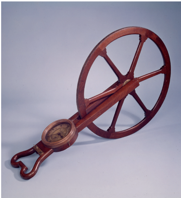
FIG. 416. A TYPICAL ENGLISH PERAMBULATOR WITH A SINGLE STOCK, CIRCUMFERENCE OF 8.25 FEET. Two silvered brass dials record distances in increments of furlongs and poles on one and miles on the other. It was made in London by Thomas Heath and Tycho Wing sometime between 1751 and 1773.
