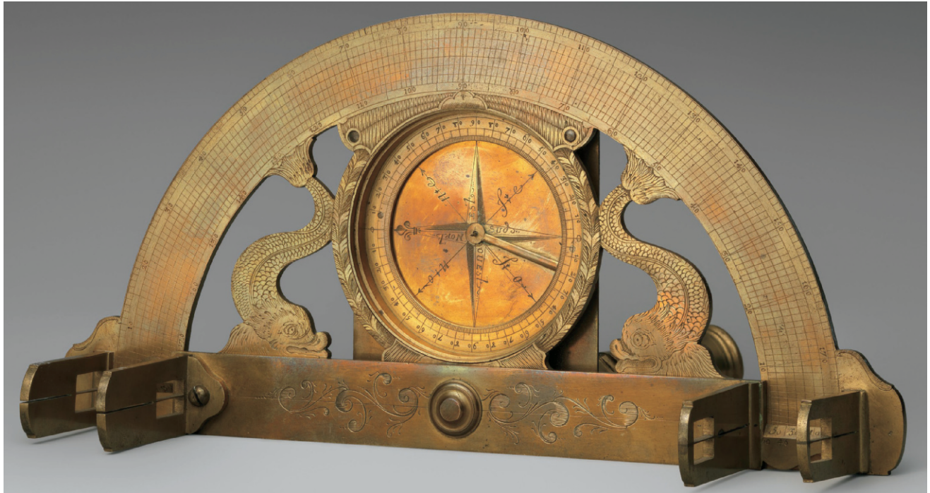
FIG. 407. BRASS GRAPHOMÈTRE BY MICHAEL BUTTERFIELD (PARIS, CA. 1700). Note the transversal scale applied to the instrument's entire arc; the main division of the arc reads to 1^\circ , the transversal to 10' of arc.
