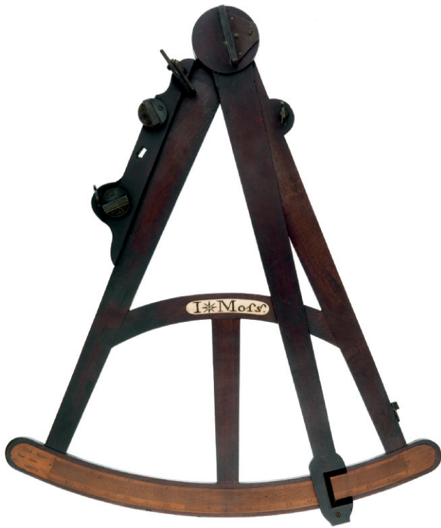
FIG. 403. PEAR-WOOD FRAME OCTANT WITH BRASS FITTINGS BY BENJAMIN COLE, CA. 1750. The octant has a brass stop on the index arm moving over an inlaid boxwood transversal scale.
