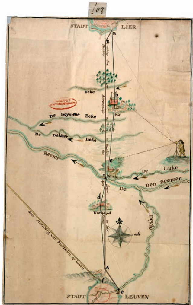
FIG. 603. JACOBUS THOMAS ROELANTS, MAP OF THE REGION FROM LIERRE TO LOUVAIN, 1734. The map incorporates an image of a civilian geometer-engineer using the triangulation method to determine the meridian line along which the road between the two cities is to be built. Manuscript, ink and watercolor on paper. Size of the original: 42.0 × 27.3 cm. © National Archives of Belgium (Cartes et plans manuscrits, Première Série, inv. No. 207).
