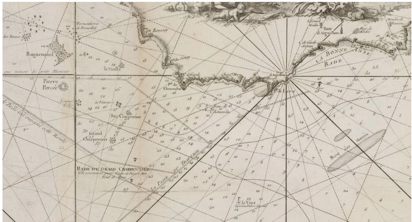
FIG. 591. DETAIL FROM MICHEL MAGIN, CARTE GÉOMÉTRIQUE DE L'ENTRÉE DE LA RIVIERE DE LOIRE , 1757. Engraved map, ca. 1:28,500. According to the author, this chart was one of the first to allow its user to function as a pilot in entering the estuary of the Loire. Magin incorporated one leading line, or line of alignment, on the chart for the navigator, using the two Tours d'Aiguillon as guides to enter safe waters, a representational device that was both modern and
