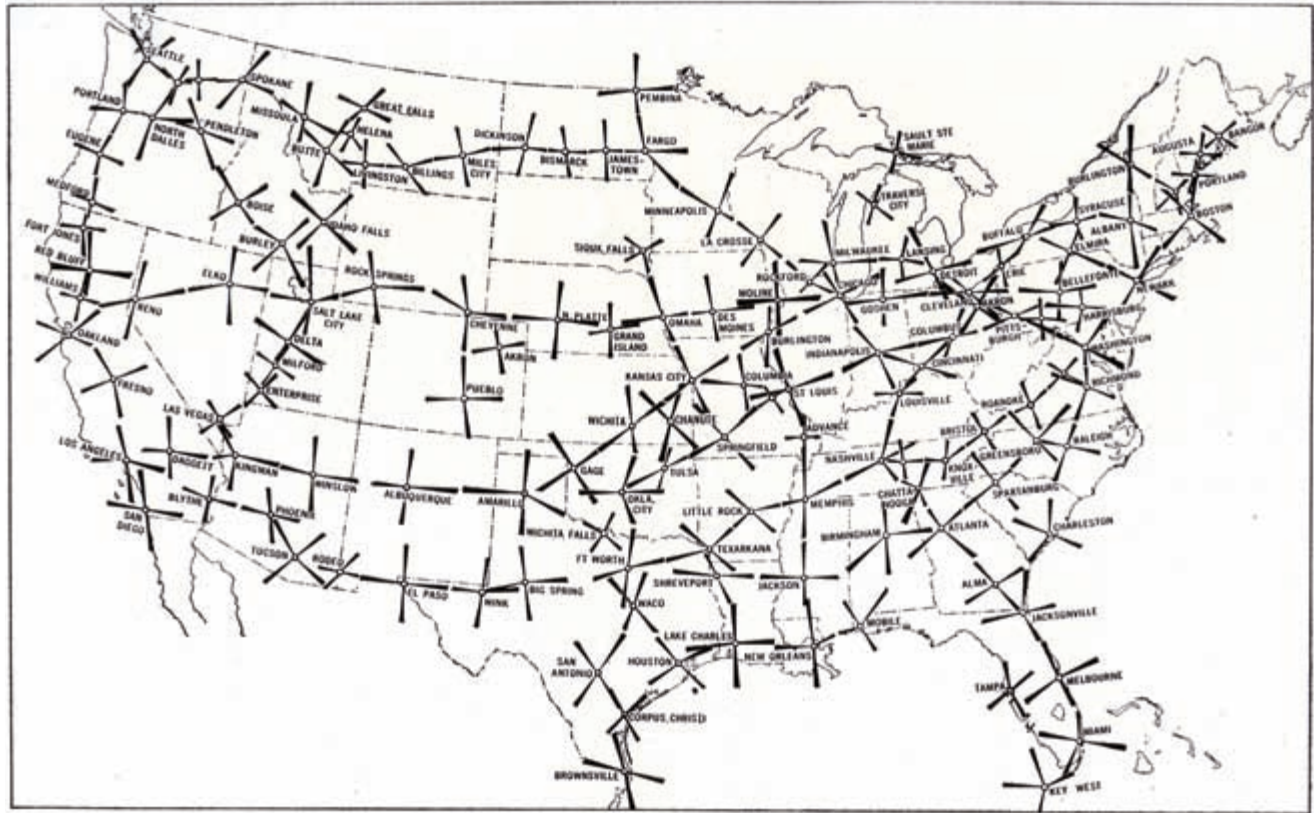
FIG. 625. THE RADIO RANGE SYSTEM OF THE DEPARTMENT OF COMMERCE, 1939. U.S. Department of Commerce, lithograph. The American radio range system, consisting of series of four-course line-of-sight radio transmitter installations, greatly aided air navigation since it required only the use of a compass, radio receiver, radio range network chart, altitude data, and airfield locations.
