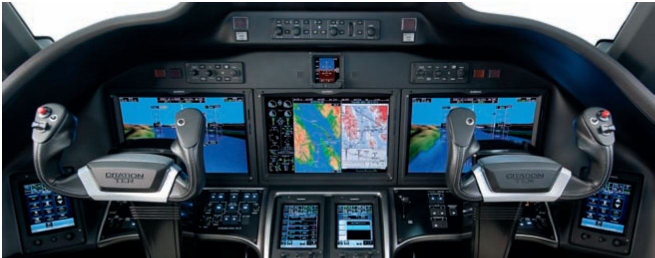
FIG. 629. COCKPIT OF CESSNA CITATION TEN BUSINESS JET. View of a typical aircraft electronic flight deck instrument display panel ENC showing approach to Juneau airport.
