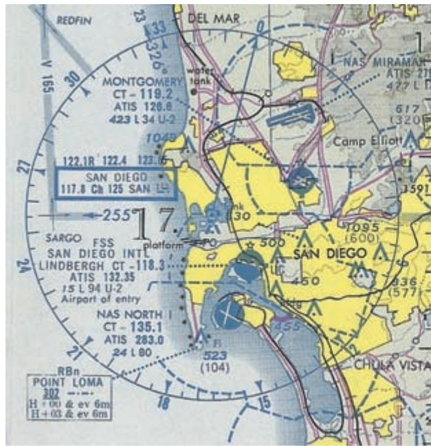
FIG. 627. DETAIL OF SAN DIEGO FROM LOS ANGELES, SECTIONAL AERONAUTICAL CHART, AND PHOTOGRAPH OF SAN DIEGO MISSION BAY VORTAC INSTALLATION. The chart (left) is on a Lambert conformal conic projection at 1:5,000,000 (15th ed., 15 August 1974) and shows a compass rose symbol with the system of radio aids to navigation that were used during the last half of the twentieth century to determine an aircraft's geographical positions
