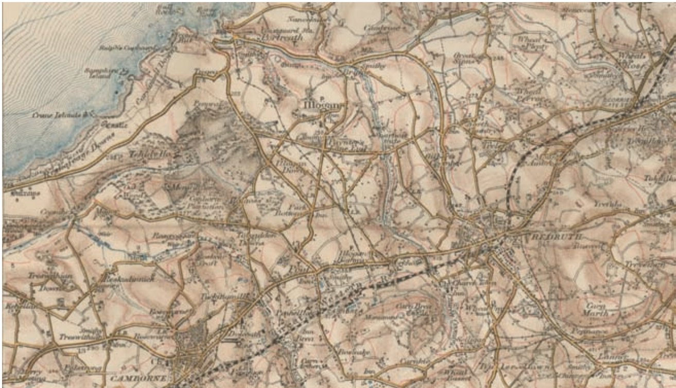
FIG. 636. DETAIL OF AN ORDNANCE SURVEY THIRD SERIES MAP SHEET ( FALMOUTH ), 1900. Sheets 352, 359 at a scale of 1:63,360. The map shows the combination of hachures, contours, and spot heights used to depict relief. The use of symbols for churches, windmills, and other prominent
