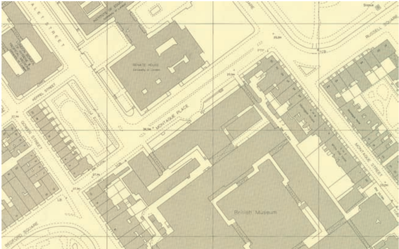
FIG. 639. DETAIL FROM AN EARLY 1:1,250 MAP PRODUCED DIGITALLY BY THE ORDNANCE SURVEY, 1972. The map showing the British Museum, London, was digitized using a Ferranti Freescan Digitizer, processed using Ordnance Survey software, and plotted by an EP 138 Automatic Light Spot Projector on a Ferranti master plotter. The plotter took two hours and forty-five minutes to complete the job. The Ordnance Survey was keen to demonstrate the flexibil-
