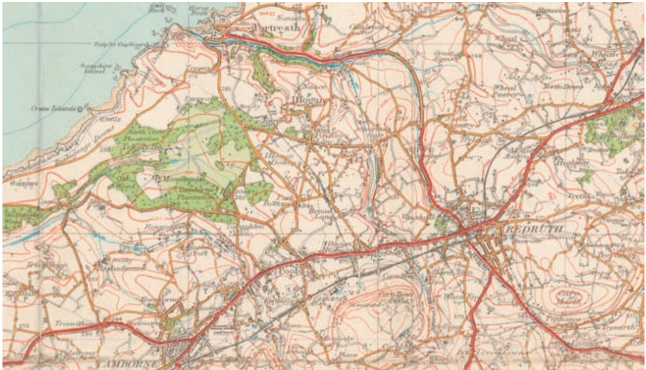
FIG. 637. DETAIL OF AN ORDNANCE SURVEY POPULAR SERIES MAP SHEET ( LAND'S END & LIZARD ), 1928. Sheet 146 at a scale of 1:63,360. The Popular Edition used only contours and spot heights for relief depiction and included a new road classification scheme.
