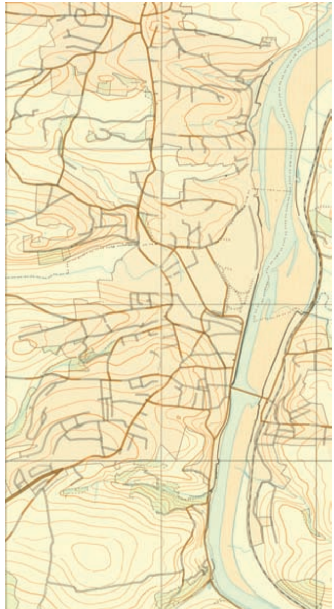
FIG. 638. DETAIL FROM AN EXPERIMENTAL TOPOGRAPHICAL MAP OF THE BIDEFORD AREA AT A SCALE OF 1:25,000. The map (sheet SS42) was produced by the Experimental Cartographic Unit of the Ordnance Survey using experimental generalization techniques. Though technically impressive for its date, the OS abandoned the automatic generalization of large-scale data to produce derived scales on the grounds of cost.
