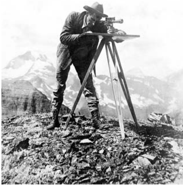
FIG. 722. SURVEYOR FROM THE U.S. GEOLOGICAL SURVEY. Herbert "Shortie" Clark using a plane table with telescopic alidade in the Rockies. Image courtesy of the U.S. Geological Survey.
