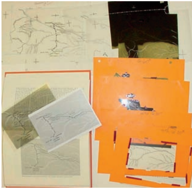
FIG. 718. STAGES OF MAP PRODUCTION. Shown here (clockwise from upper left): pen-and-ink drafting with stick-up lettering on mylar film; film negatives for making block-out positives; punch-registered film negatives and positives with photographic tint screen percentages and angles marked on orange masking paper; photographic composites on paper and film; and the printed map illustration in the book. Original map is illustrated in William Y. Chalfant, Cheyennes and Horse Soldiers (Norman: University of Oklahoma Press, 1989), 117. Image courtesy of Kansas University Map Associates.
