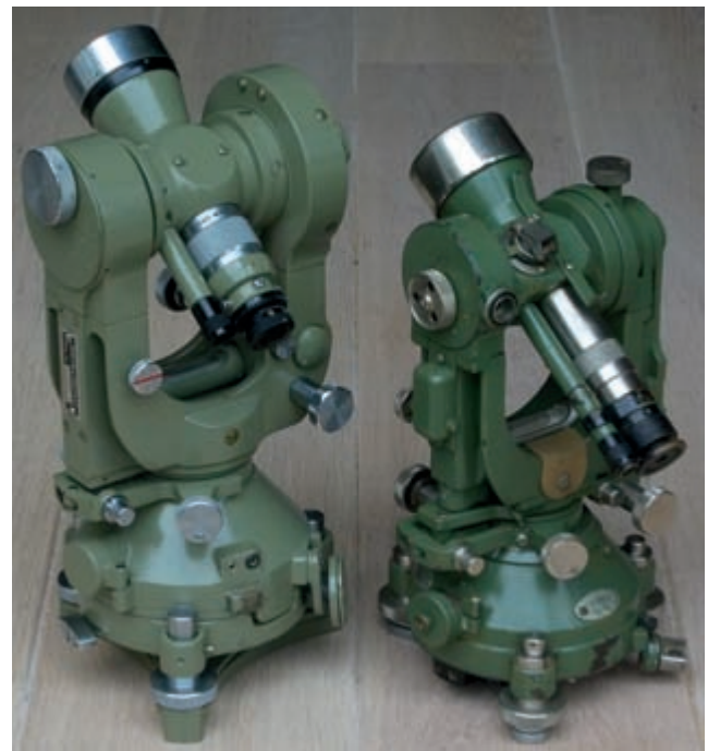
FIG. 753. TWO WILD T-2 THEODOLITES. A 1970s model (left) and an early 1929 model (right). Image courtesy of Nicolàs de Hilster.
