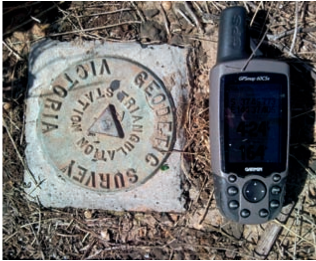
FIG. 774. AUSTRALIAN BRASS GROUND MARKER AND GPS UNIT. Marker is at the summit of Mount Cottrell in Melton.
