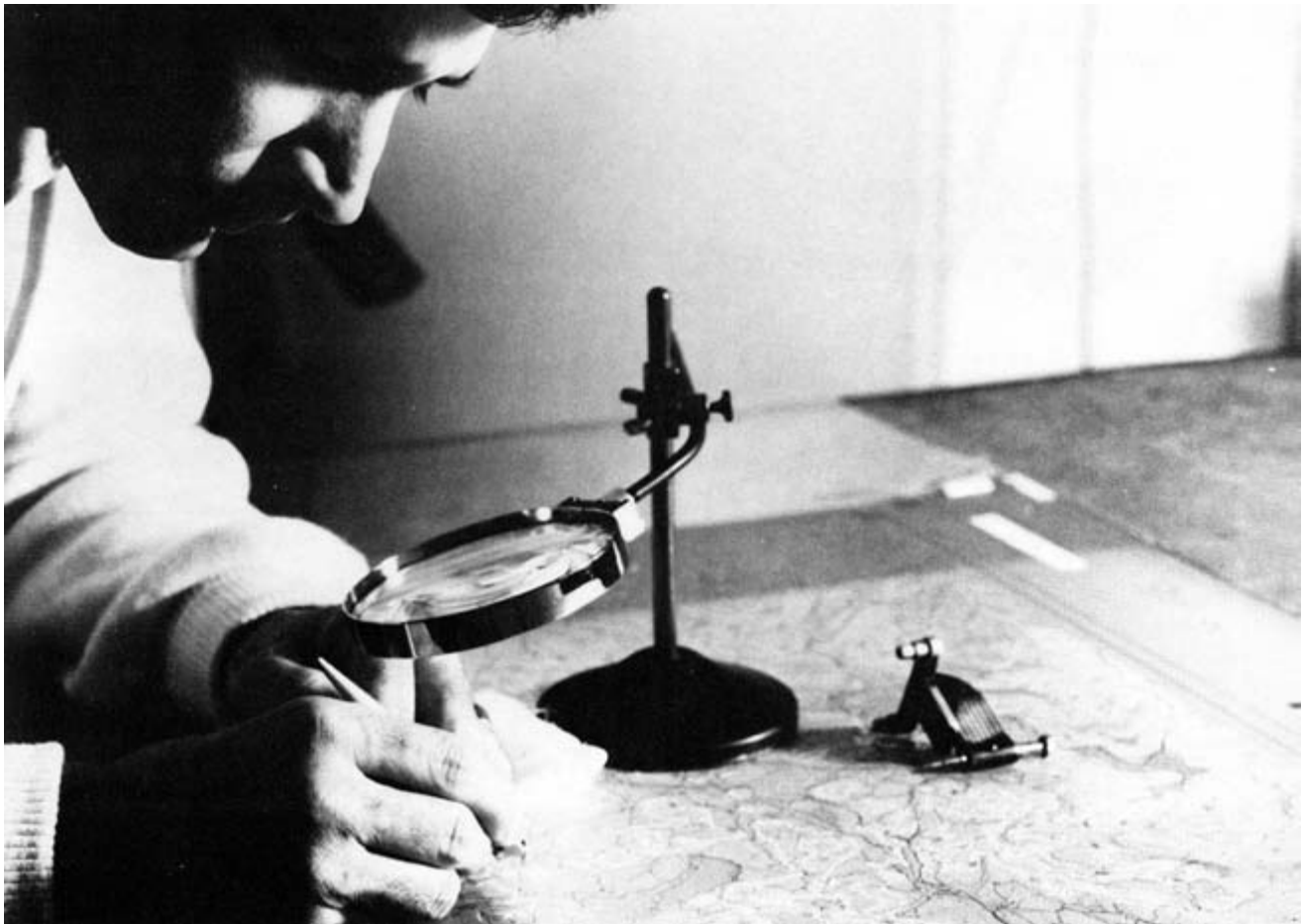
FIG. 719. MAP SCRIBING. Contour lines for a topographic map are being scribed by following a photographic guide image printed on scribecoat with a handheld pen-style scribing tool, while a rigid graver rests nearby on its side, ready to be picked up and pushed across the scribecoat removing lines of
