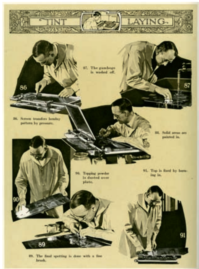
FIG. 714. STEPS IN ADDING BEN DAY TINTS TO A PHOTOENGRAVING. Size of the original: 21.5 × 15.7 cm. From Flader 1927, 126.
