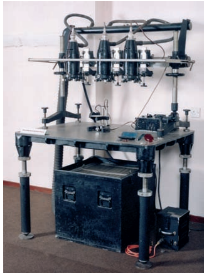
FIG. 684. WILLIAM-ROSS MULTIPLEX MARK 1 WITH THREE PROJECTORS. The development of the multiplex plotter permitted low-cost photogrammetry and was widely used between the 1930s and 1970s. This particular instrument was made by the Williamson Company in Britain. Image courtesy of the Defence Surveyors' Association, U.K.
