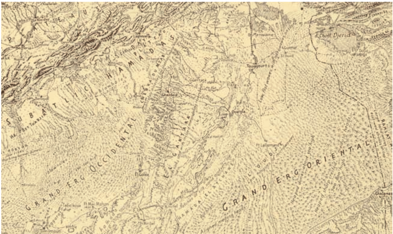
FIG. 721. DETAIL FROM THE LANDFORM MAP OF NORTH AFRICA, 1952, BY ERWIN RAISZ. Trimetrogon photography provided the chief source for this map, enabling Raisz to portray Saharan dune systems and desert landforms in intricate detail. Note the use of descriptive terms and the
