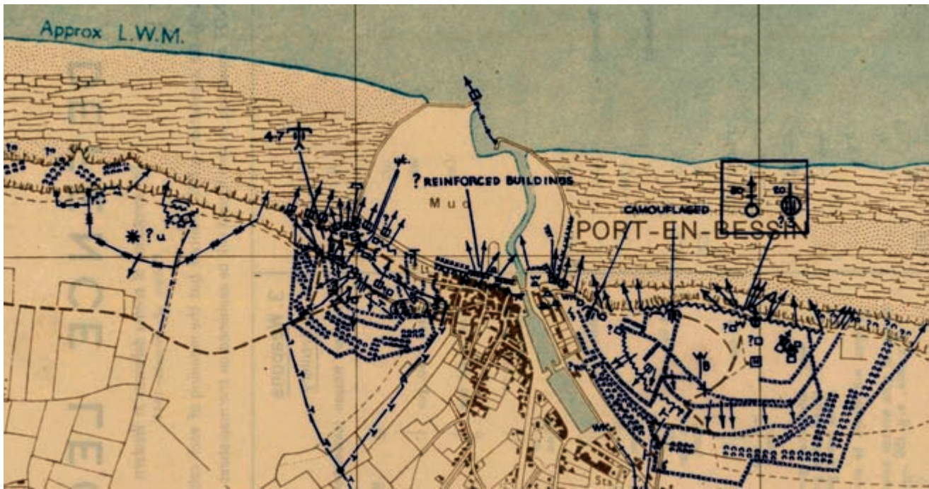
FIG. 691. DETAIL OF A BABY BENSON. Map shows the beach defenses at Port-en-Bessin on the Normandy coast. The information on this map ( Defences , GSGS 4490, sheet no. 81, May 1944) is nearly all derived from aerial photography. Benson was the name given to the secret 1:25,000-scale maps
