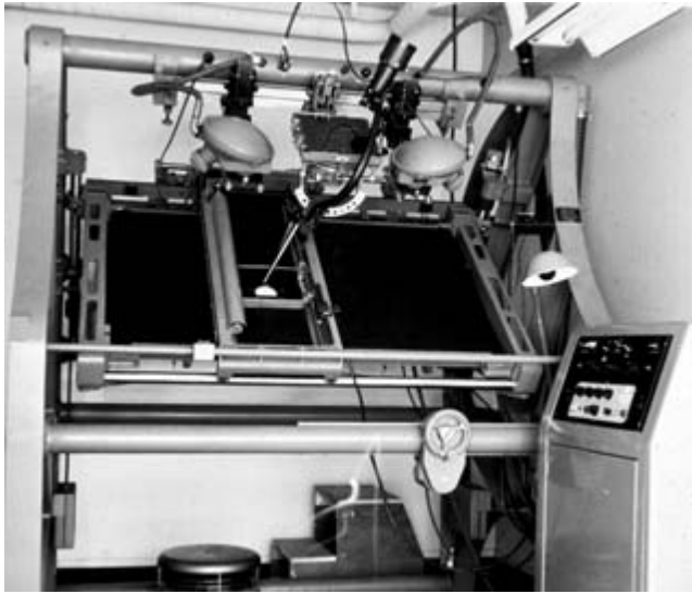
FIG. 708. KELSH T-64 ORTHOPHOTO EQUIPMENT, CA. 1964. The T-64 orthophotoscope was designed and built in 1964 by Russell K. Bean at USGS. Shown here is the first orthophotoscope in Menlo Park, California, used to produce orthophotoquads. Image courtesy of the U.S. Geological Survey.
