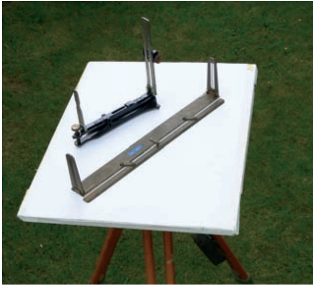
FIG. 724. WILD PLANE TABLE WITH SIMPLE ALIDADE AND INDIAN CLINOMETER. Image courtesy of Peter Collier.
