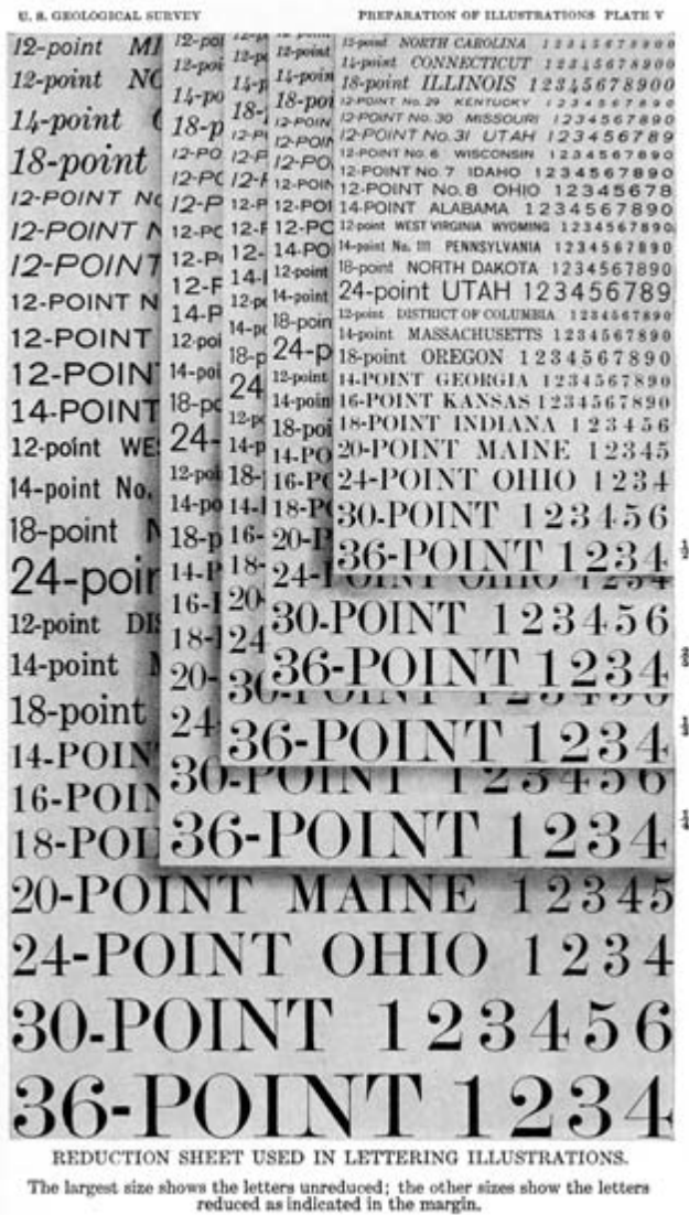
FIG. 710. TYPE REDUCTION SHEET USED FOR DESIGNING U.S. GEOLOGICAL SURVEY ILLUSTRATIONS. Size of the original: 18.7 × 11.3 cm. From John L. Ridgway, The Preparation of Illustrations for Reports of the United States Geological Survey with Brief Descriptions of Processes of Reproduction (Washington, D.C.: Government Printing Office, 1920), facing 54.
