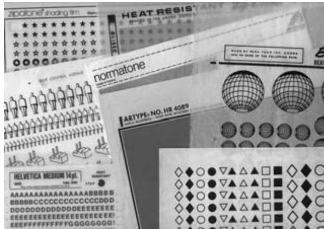
FIG. 716. DIFFERENT BRANDS OF RUB-DOWN AND STICK-UP LETTERING AND SYMBOLS. These were staples of map production for photography from the 1920s through the 1970s, after which their use declined. Image and permission courtesy of George F. McCleary, Jr.
