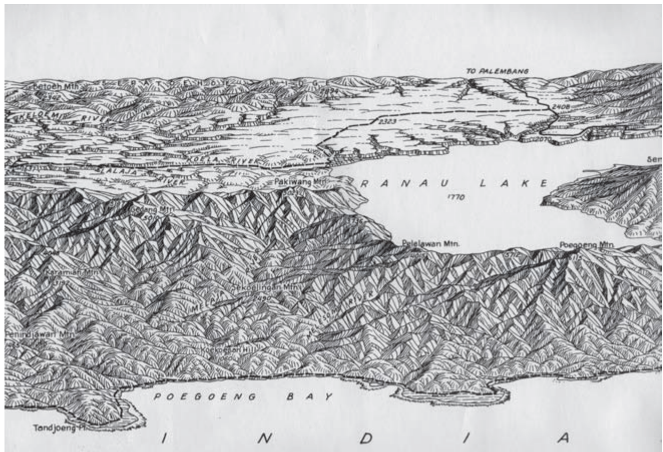
FIG. 937. DETAIL FROM AN ISOMETRIC TERRAIN DIAGRAM, LAKE RANAU AREA OF SOUTHERN SUMATRA. As with all types of parallel projection, objects drawn with an isometric projection did not appear larger or smaller as they
