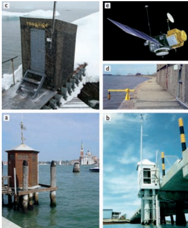
FIG. 968. TIDE GAUGES FOR MEASURING SEA LEVEL FROM AROUND THE WORLD. (a) Float and stilling well gauge at the Punta della Salute, Venice (photo credit: P. A. Pirazzoli); (b) acoustic gauge at Kiribati, South Pacific (photo credit: National Tidal Centre, Australia); (c) float gauge at Vernadsky, the site of the longest sea level record in Antarctica (photo credit: British Antarctic Survey); (d) radar tide gauge installation at Liverpool, U.K. (photo credit: National Oceanography Centre Liverpool); and (e) TOPEX/Poseidon radar altimeter satellite. This composite figure was constructed by Lea Crosswell of the Commonwealth Scientific and Industrial Research Organisation (CSIRO), Australia, and has been copied with permission from John A. Church et al., eds., Understanding Sea-Level Rise and Variability (London: John Wiley & Sons, 2010), 7 (fig. 1.5). Permission courtesy of John Wiley & Sons, Inc.
