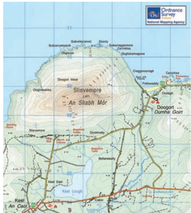
FIG. 1011. DETAIL FROM ORDNANCE SURVEY OF IRELAND DISCOVERY SERIES, 1:50,000, 1994. Overhauls of map series during the last quarter of the century offered opportunity to integrate photogrammetric and digital techniques into the production flow line as in this example, Straith Eolais: Maigh Eo (sheet 22) published by the OSI. Fine photogrammetric contouring combined with layer tinting made this an attractive topographic map series.
