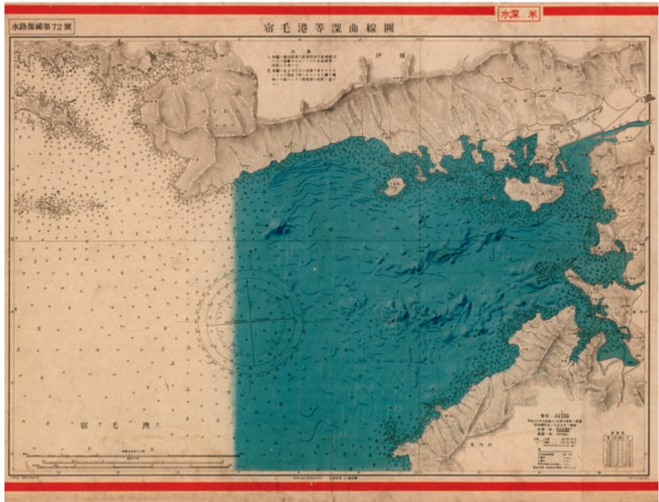
FIG. 929. SUKUMO-WAN TŌSHINKYOKUSEN ZU 宿毛湾等深曲線圖 (DEPTH CURVE CHART FOR SUKUMO HARBOR AND VICINITY), 1939. One of the two trial sheets to publicize Tanaka's relief contour method. Red borders on the top and bottom indicate the chart was secret at one time. The
