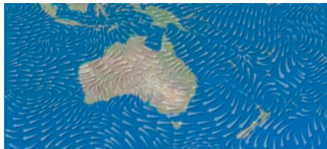
FIG. 962. AN AUTOMATED METHOD FOR FLOW MAPPING. Depiction of wind direction and magnitude over Australia. The method utilizes an energy measure (lower energy equates to higher quality) to improve the position of flow lines. Size of the original: 8 × 17.8 cm. From Turk and Banks 1996, 458 (fig. 7). © 1996 Association for Computing Machinery, Inc. Reprinted by permission.
