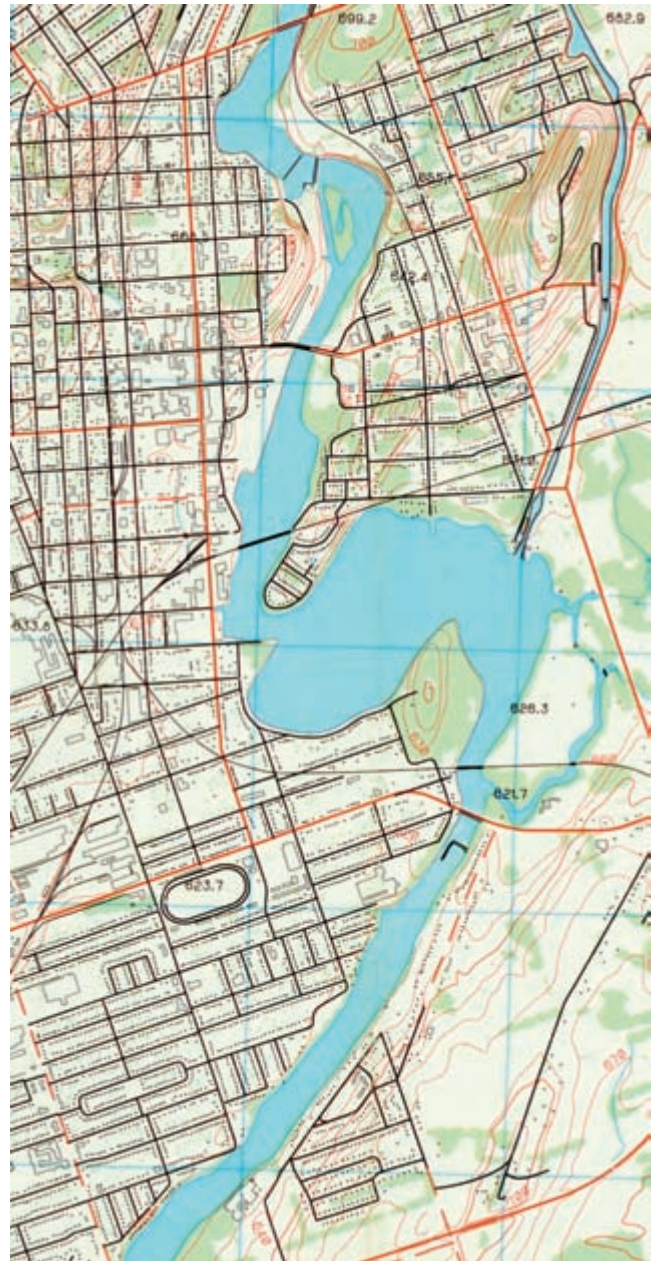
FIG. 981. DETAIL FROM AN EXPERIMENTAL MAP OF PETERBOROUGH, ONTARIO, CANADA, 1:25,000, NOVEMBER 1971. The map was produced within the Photogrammetry Office, Department of Transportation and Communications, Ontario, in cooperation with the Department of Energy, Mines and Resources, Ottawa, Canada. It claimed to be “untouched-by-human-hands” with the exception of the peel coats used for the areas covered by vegetation and water bodies.
