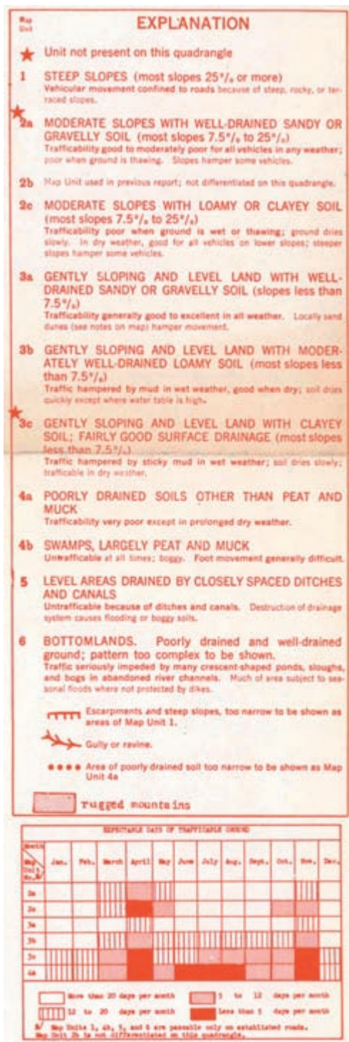
FIG. 939. KEY TO TRAFFICABILITY MAP SHOWN IN FIGURE 938. Eleven terrain unit types were identified and explained with the aid of this key. A table also provided the number of days in every month that each terrain type would be trafficable, and climate data were also provided by the Weather Division, Headquarters, Army Air Forces and the U.S. Weather Bureau. Size of detail: 25 × 8.2 cm. Image courtesy of Alastair W. Pearson.
