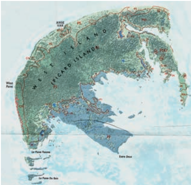
FIG. 980. DETAIL FROM ALDABRA ISLAND (WEST SHEET), CA. 1:25,000, 1969. An experimental photomosaic produced by the Directorate of Overseas Surveys (from aerial photography flown June 1960) for the Royal Society's expedition 1967–68. Photomapping became a cost-effective method of mapping remote and inaccessible areas.
