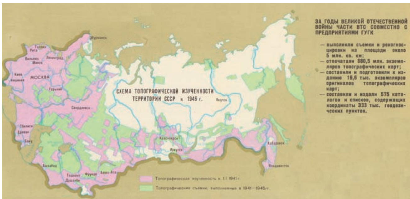
FIG. 1019. TOPOGRAPHIC MAPPING OF THE SOVIET UNION BY 1946. The legend categories are: topographic investigation by 1 January 1941 and topographic surveys performed from 1941 to 1945. The text to the right lists achievements by the VTS and the GUGK during the Great Patriotic War: they made surveys and did reconnaissance in an area of about 5 million square kilometers, published 880.5 million
