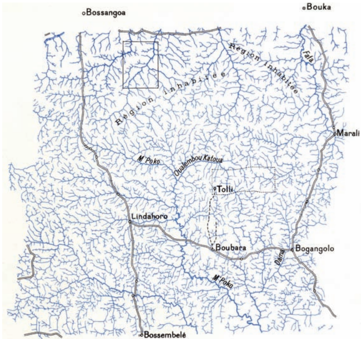
FIG. 999. DETAIL FROM SKETCH MAP AT 1:1,000,000 OF THE UBANGUI DISTRICT, 1946. Covering the same area as figure 998, this map was compiled from aerial photography and illustrates the major improvement in accuracy and data content once aerial photography entered widespread use in Africa.
