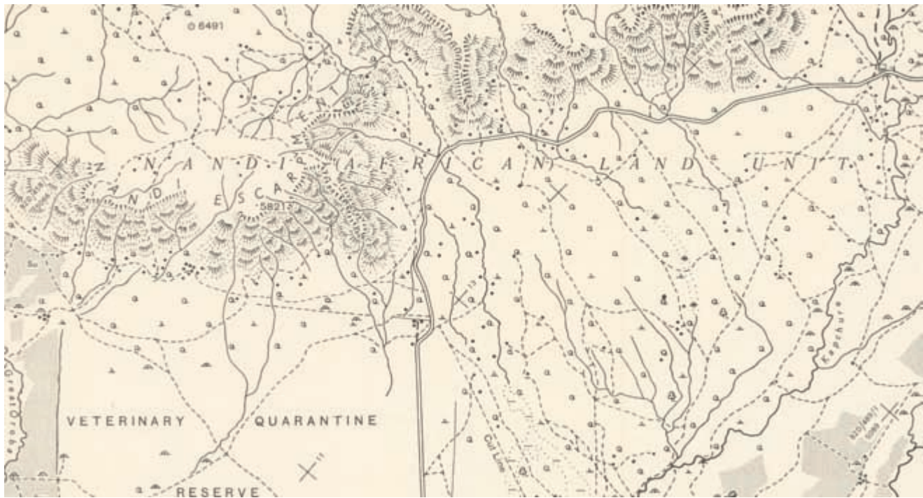
FIG. 995. DETAIL FROM 1:50,000 PRELIMINARY PLOT, KENYA, 2d ED., 1954. Sheet A-36/F-I-NW. These sheets were produced very rapidly by radial line methods, but lacked vertical control for contouring, hence the use of hachures to depict relief.
