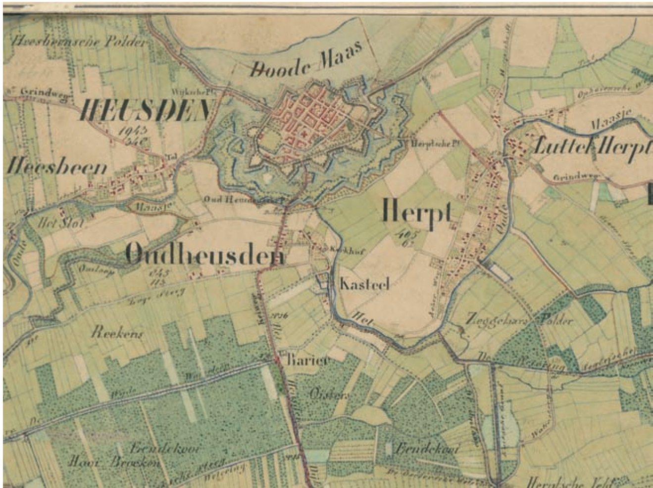
FIG. 975. TERRAIN SURVEY (CALLED A “MINUTE”), 1:25,000. Before the use of aerial photography, topographic reconnaissance was surveyed and drawn on the basis of reduced cadastral maps. The drawing of the terrain details was performed in the field and the coloring done during the night’s
