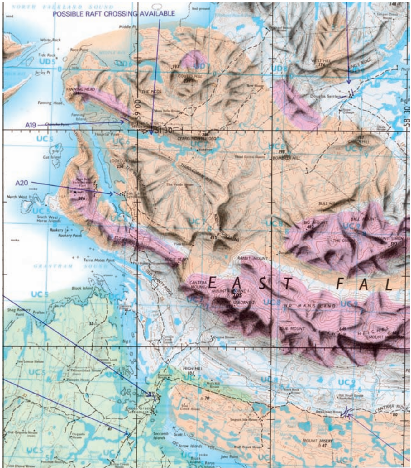
FIG. 940. DETAIL FROM FALKLAND ISLANDS ROYAL ENGINEERS BRIEFING MAP , 1982. This map (GSGS 5453 Edition 3-GSGS, 1:250,000) was produced by the headquarters engineer-in-chief and the Forty-Second Survey Engineer Regiment and was based on the British Royal Marines and Royal Engineers reconnaissance and from information gleaned through interviewing over forty Falkland Islanders. Studies conducted by the British Antarctic Survey and geolo-
