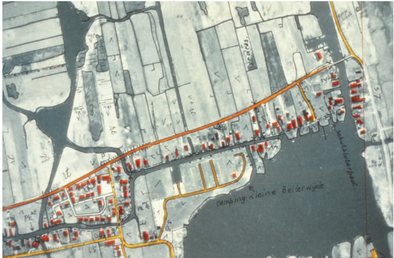
FIG. 976. ANNOTATED PHOTOMAP, 1:10,000. This became the source for scribing the topographic basemap, 1:10,000 (1930–2005).
