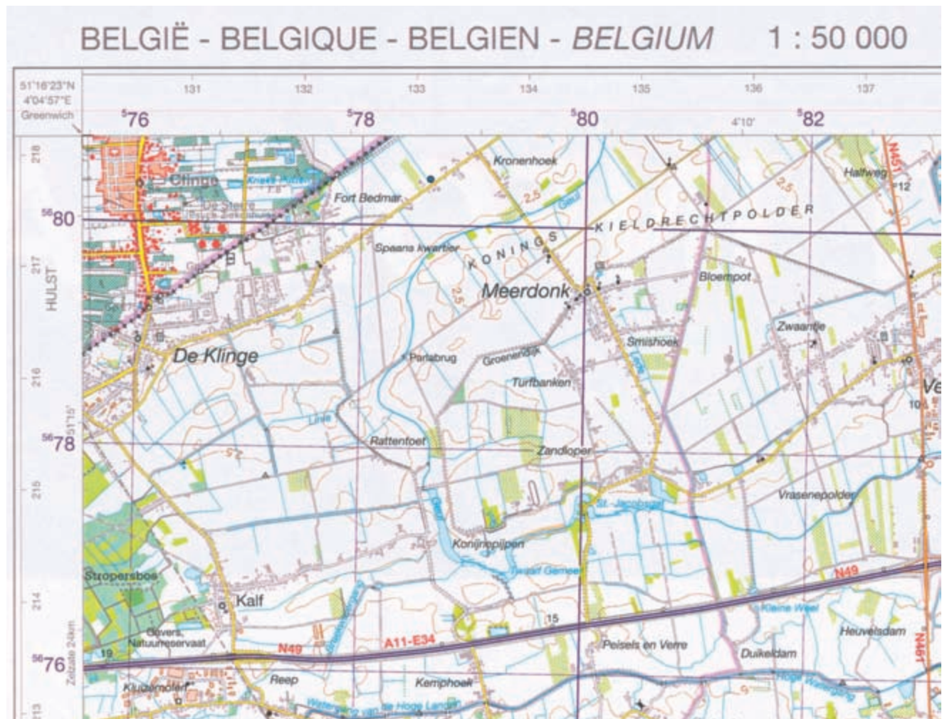
FIG. 1013. DETAIL FROM BELGIAN 1:50,000 MAP, 2000. Antwerpen (sheet 15) published by the Institut géographique national, Brussels. Though at the administrative heart of the European Union, the sheet demonstrates the lack of standardization in West European topographic mapping. The Dutch specification of mapping is adopted in the top left corner for
