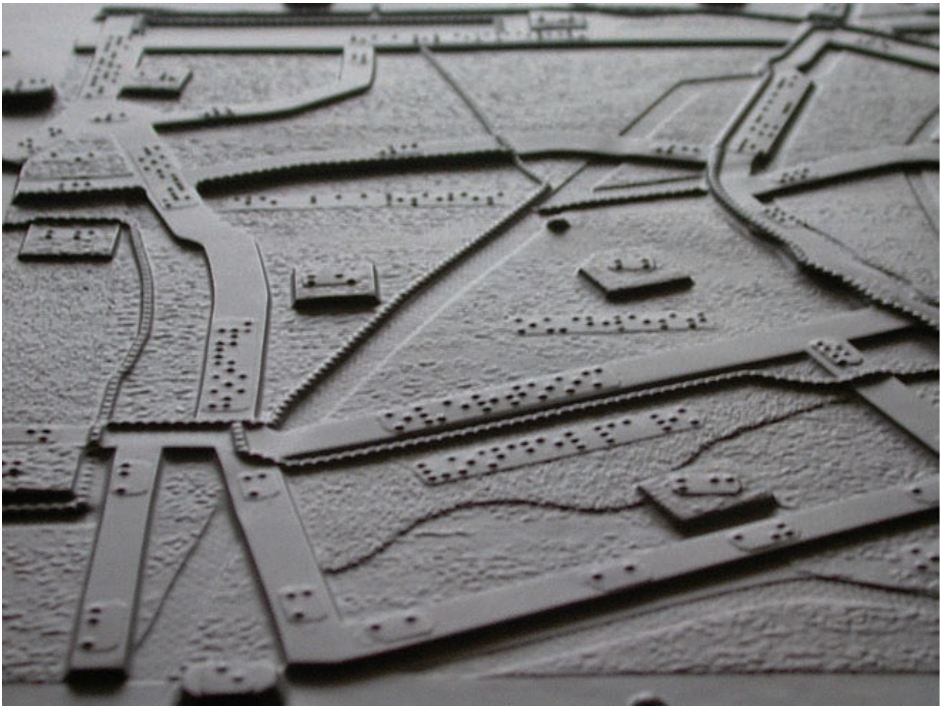
FIG. 926. PORTION OF A LARGE-SCALE THERMOFORMED CITY PLAN OF AMSTERDAM. The map shows major routes, street names, waterways, and points of interest and is part of a ring-bound hardcover atlas with detachable sheets.
