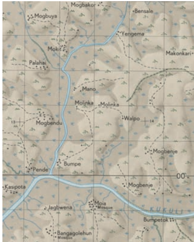
FIG. 996. DETAIL FROM 1:50,000 MAP OF SIERRA LEONE, BAUYA SHEET, 1964. Sheet 75. These maps lacked height information for contouring but relief was shown using hill shading derived from inspection of the aerial photographs. Size of the entire original: 78.5 × 58.8 cm; size of detail: 13.8 × 11.1 cm. Image courtesy of Peter Collier.
